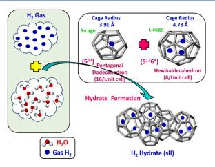
Figure 11. Schematic representation of  $H_2$  hydrate (sII) formation. Sixteen pentagonal dodecahedron ( $5^{12}$ ; S-cage) cages and eight hexacaidecahedron ( $5^{12}6^4$ ; L-cage) cages combine in order to form a single unit cell of sII hydrate. The multiple occupancy of L-cages results in increasing the  $H_2$  storage capacity of the hydrate.
