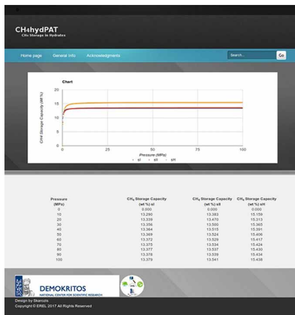
Figure 13. Snapshot of the third page of the web-based calculator. Example of results (given as a figure and tabulated) for case A with option of examining the comparison of the three structures. Parameters used: pure CH 4 hydrate at T = 270 K.
